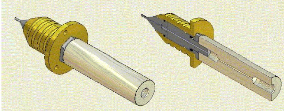
This system was designed to improve ultrasonic surface contact with the tube material.
