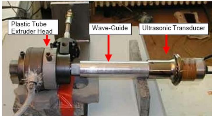
The transducer must have a way to make strong and solid coupling to the extruder internal or external die. We normally use a wave-guide as a coupling interface. We can put water jackets (not shown) on the wave-guide to prevent excessive heat build-up to the transducers.
